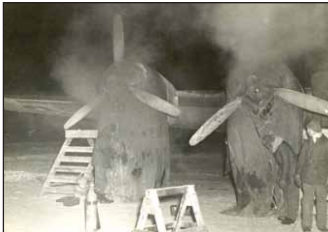
As a part of the test regimen, personnel experimented with different ways to warm the engines. Here insulated canvas covers enclosed gas-fired burners.
