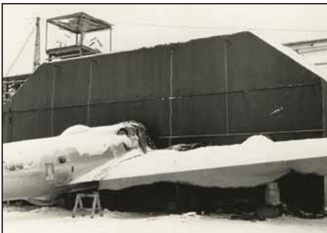
Without a completed hangar, in the winter of '40-'41, maintenance was performed with the aid of a heated "nose shelter" constructed locally.
